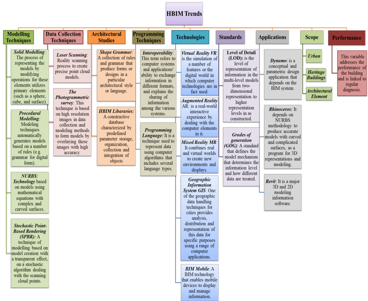
Figure 13 HBIM Integration Trends based on the study made by (Khalid A. Hussein, 2020).
