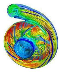
Figure (1) shows the distribution of air inside the pump
