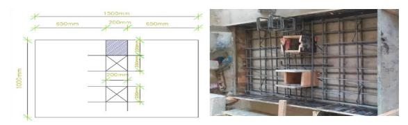
Fig. 2: Layout of slab with two openings
