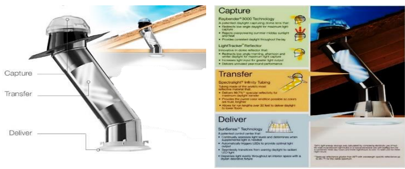
Figure 17 Components of natural tubular lighting units
