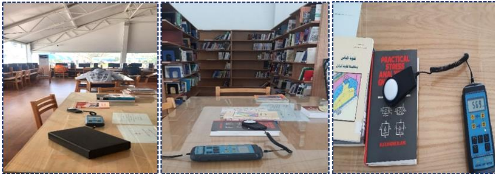
Figure 21 Different measurements within the viewing area showing the achievement of the required levels of natural light by "DIGITAL LIGHT METER".
